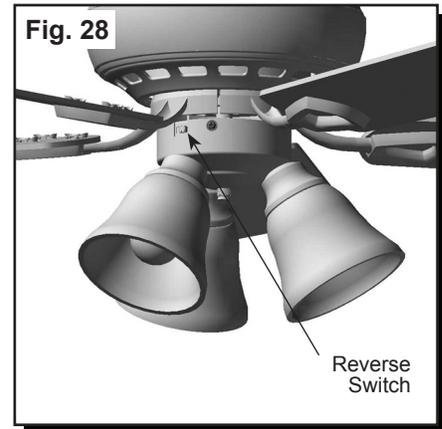
29. **In warmer weather**, push the reverse switch left, which will result in downward airflow creating a wind chill effect (Fig. 29).
