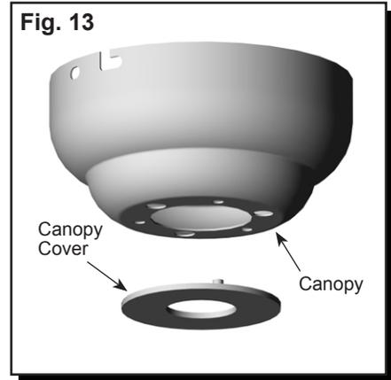
14. Align the canopy with the closemount screw holes in the top of the motor housing. Secure the canopy to the top of the motor housing with the closemount screws and spring washers into the top of the motor housing (Fig. 14).
